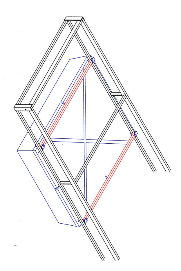
PLACE DOCK FRAME ON FLOAT, THEN HOOK BRACKET OVER LOWER FRAME TUBE AND PUT BOLT THROUGH BRACKET INTO SLOT IN FLOAT AND ATTACH USING WASHER AND NUT. DO THIS ON ALL FOUR CORNERS OF EVERY FLOAT.
